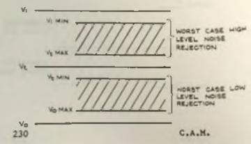
Even if these last provisos are kept in mind, such a specification, and therefore such a performance guarantse from the integrated circuit supplier, is quite inadequate in practical cases. This is because two other failure modes are common with present integrated circuit designs.
