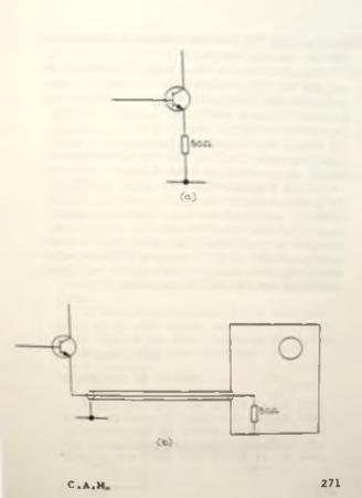
across the SO ohm resistor is displayed at the oscilloscope.
