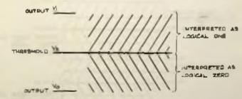
The noise rejection is commonly described as the difference between the minimum possible Vt and the maximum possible VO for circuits which are operating within specification for noise rejection at the low logic level, and the difference between the maximum possible Vt and the minimum possible V1 for noise rejection at the high logic level. Put mathematically, noise rejection is ( Vtmin - VOmax ) and ( Vlmin - Vtmax).
