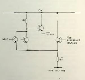
No current except the small base drive current to the output transistor flows in R1, and the NOR output stands at the high level of one diode drop (Vbe) below OV. So a low input causes a high output. As the input voltage rises above Vbb, the current I is deflected down the left hand path, and causes a drop across R. The result is that the NOR output drops to the correct low logic level.
