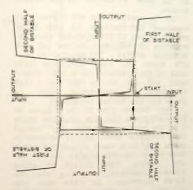
in a noisy environment. There is a cartain pattern of random noise which will alternatively move the bistable to one side and the other of its metastable state, but not far enough for it to move to one of its two stable states.
