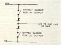
+5v, but will not prevent noise from pulling it up even higher. With the lower switch on, the circuit clamps the output down to 0v, but will not prevent noise from pulling it even lower. So in no case can noise reduce the voltage difference between the two lines and so increase the problem of discrimination by the line receiver circuit.
